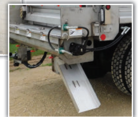
Berm chute option shown. Can be used for left or right discharge.
